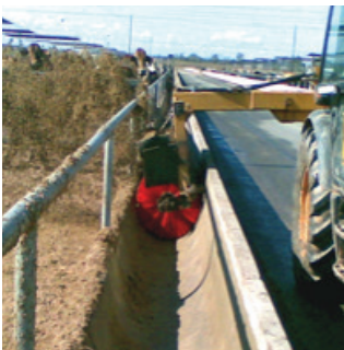
Loader too close to bunk. Swing arm not straight. Leaving feed in bunk.
