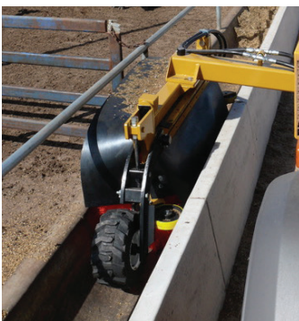
Rear guide wheel positioned correctly against the road-side wall.
